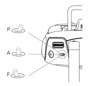
P-mode (Positioning): P-mode works best when GPS signal is strong. There are several states in P-mode which are automatically selected by the Matrice 600 depending on GPS signal strength: P-GPS: GPS is available. The aircraft uses GPS for positioning.
