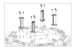
Mount the base plate of the expansion bay to the brackets by inserting and tightening eight M3x5.5 screw.
