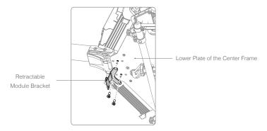
2. With the servo of the retractable module at the rear of the aircraft, insert the retractable module mounting rod into one mounting hole on the center frame, mounting holes on the retractable module and the other mounting hole on the center frame respectively. Ensure that the left retractable module is mounted on the left side of the aircraft (when viewed from the rear).
