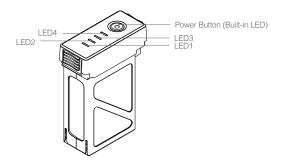
Powering On: Press the Power Button once, then press again and hold for 2 seconds to power on. The Power LED will turn red and the Battery Level Indicators will display the current battery level.
