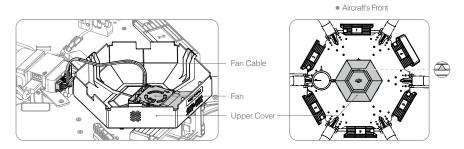
DO NOT damage the fan cable when removing the upper cover of the center frame.
