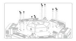
Mount the four brackets of the expansion bay to the upper plate of the center frame by inserting and tightening twelve M3×8 screws.
