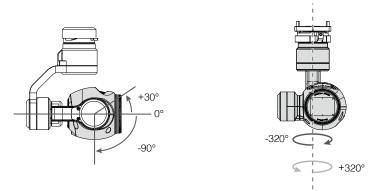
Under the default settings, turn the gimbal dial on the remote controller to tilt the camera. Note that you cannot simultaneously tilt and pan the camera in the Single Remote Controller mode. Enable the Master-and-Slave mode in the DJI GO app and set a second remote controller to Slave if you wish to tilt and pan the camera together.
