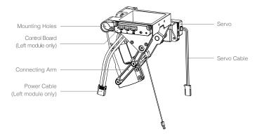
Mount the retractable module bracket to the mounting position on the lower plate of the center frame as shown below. Apply medium strength threadlocker to two M3x8.5 screws. Insert and tighten the screws.
