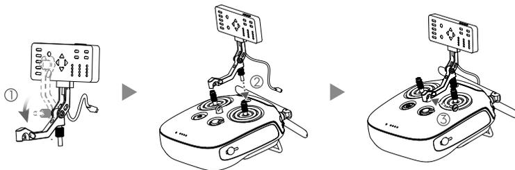
4. Tilt the Spraying Status Panel to the desired position. Adjust the antennas as shown.
